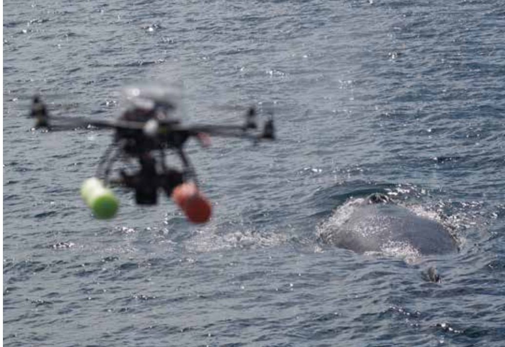
A remotely operated hexacopter or drone approaches a humpback whale in the waters surrounding Patagonia, Chile. The drone holds a petri dish, which is used to collect exhaled breath or blow samples from large whales. These blow samples are being analysed to understand the composition of the associated microbiome. This technique is being explored as a means to non-invasively assess the respiratory health of whales. Courtesy of Daniel Casado (MERI) and taken under permit MERI 1197-Feb-2017
