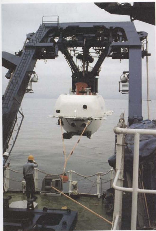
Fig. 2. Launching 'Shinkai 2000'. The submersible can be lowered into waves up to 2 m and the whole process takes about 10 minutes. Photo courtesy of Joy Colquhoun.
