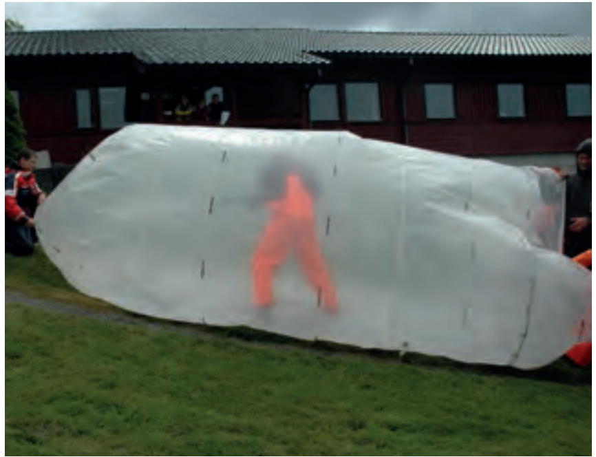
The study of giant viruses often requires the use of giant bags (mesocosms), which can be filled with seawater and studied under natural conditions. Willie Wilson and Mike Allen
