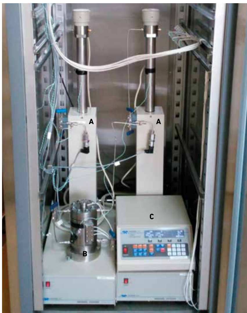
Apparatus used to conduct experiments used to study the impact of micro-organisms in swelling clays on swelling capacity and steel corrosion. Two high pressure pumps (A) control the flow of groundwater through a clay sample held in a bespoke flow cell (B). The flow cell has continuous monitoring to record changes in flow and in the force exerted by the swelling clay (C). Megan Barnett, BGS
