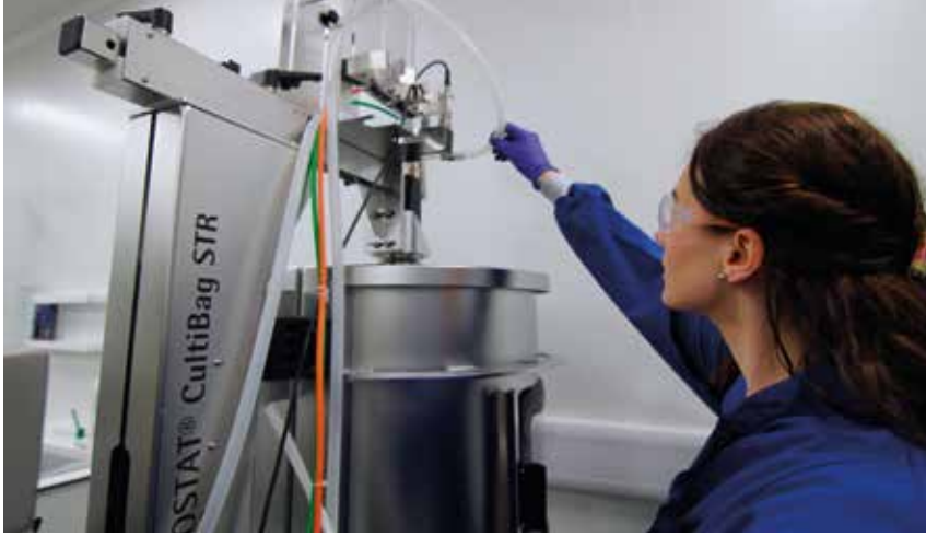
Large-scale production for commercial purposes can be carried out in 250 l bioreactors. © CPI 2018
