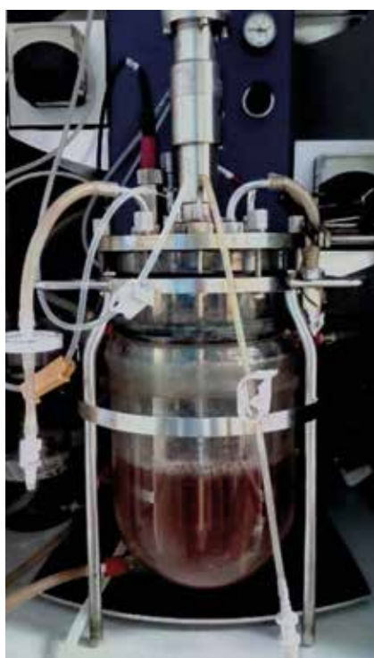
Fig. 2 Some aspects of the microbiome can be modelled by inoculating fermenter vessels with faecal samples, single isolated cultures or artificial consortia, and applying a range of analyses including transcriptomics and metabolomics to measure interactions and products. M. Perez & P. W. O'Toole
