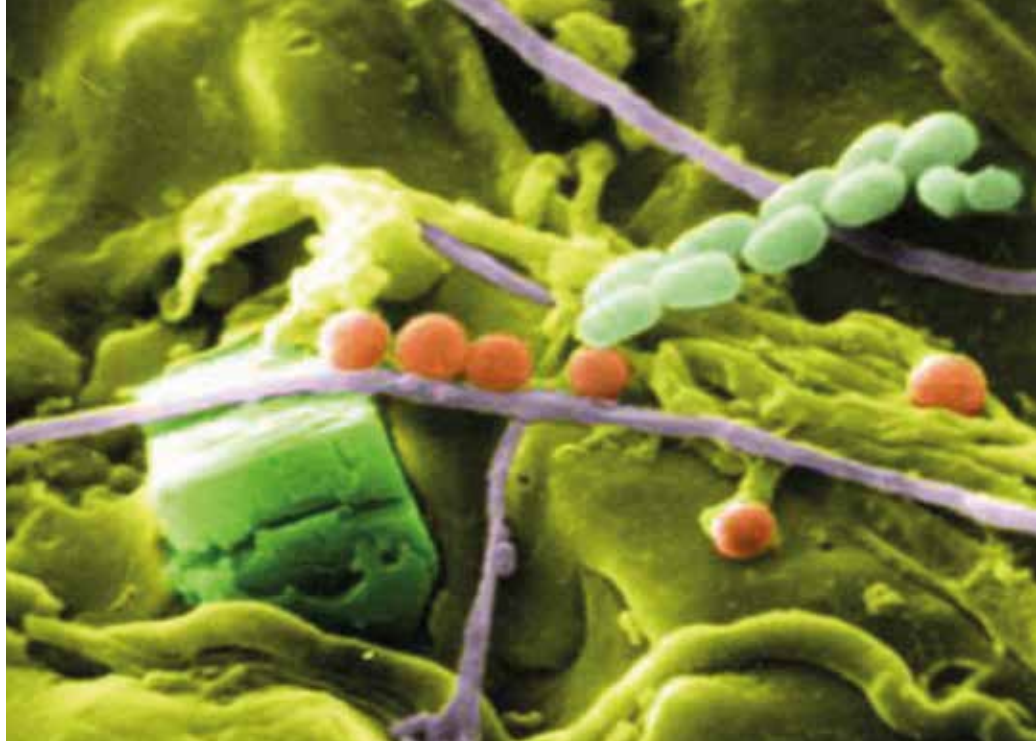
False-colour SEM image of a soil showing clays, bacteria and fungi spatially located from a soil smear.
